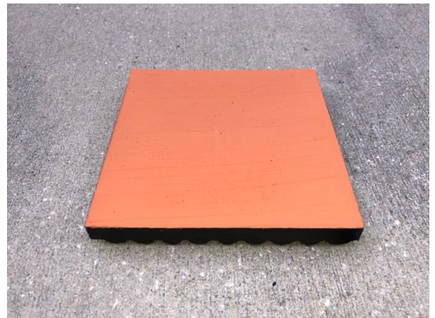
Semplastics' X-TILE™ sample made of Appalachian coal
